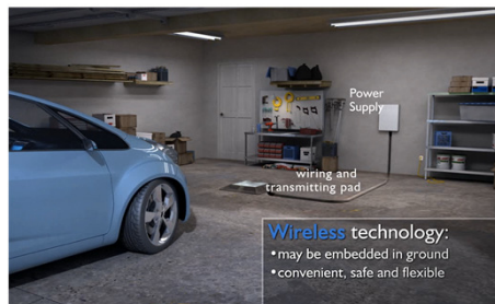
Stationary Wireless Charging
