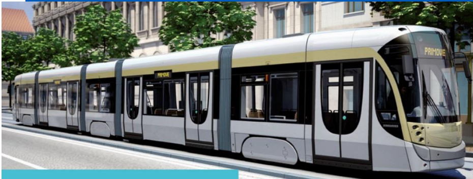
Light Rail: Continuous 270kW power, buried cables replaces catenaries
