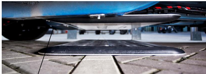
Affixed vehicle pad & Transmitter pad
